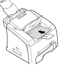
If there is any resistance and the paper does not move when you pull or if you cannot see the paper in the front output tray, continue to step 3.
